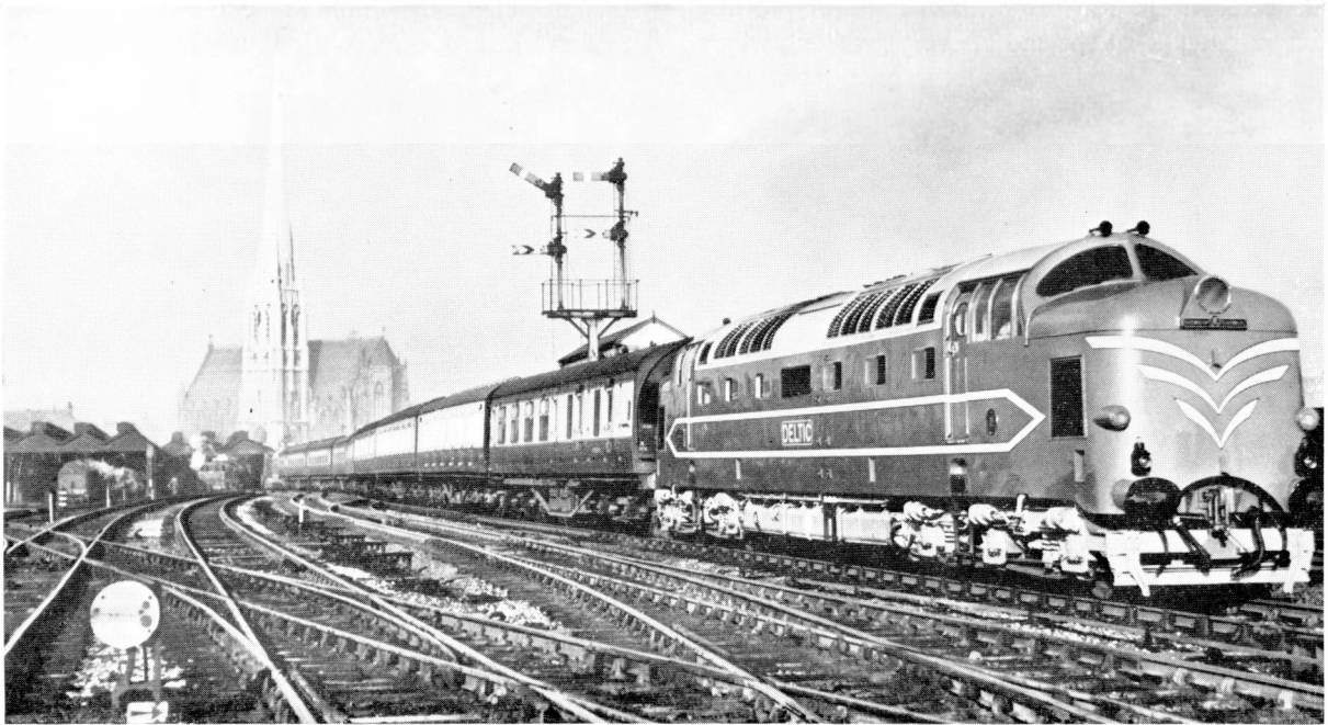
Fig. 3.—The 3,300 h.p. 'English Electric' Deltic locomotive
