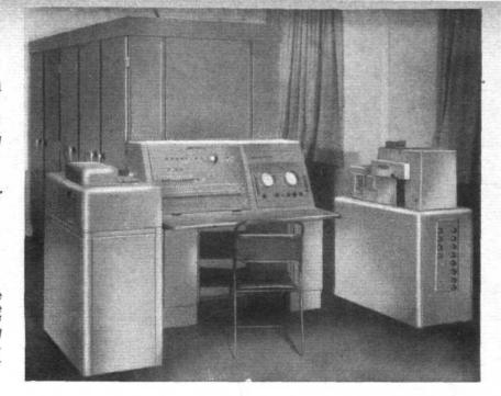
HEN, shortly after the end of World War 2, the National Physical Laboratory wished to develop an electronic calculating machine of greater potential than any built previously, they sought assistance from the English Electric Co., Ltd. Scientists and engineers from the latter co-operated with the N.P.L. to such effect that the pilot-model ACE (Automatic Computing Engine) was put "on steam" at the N.P.L. mathematics division early in 1952, since when it has proved outstandingly successful.
