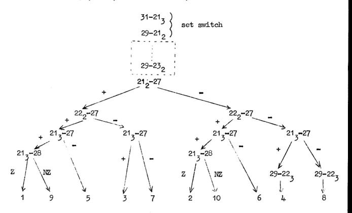
Three instructions are used to "change the points", a common 29-232 within the routine from which the several exits are required and two 29-22, instructions on the exit branches 4 and 8. TCB is assumed to be OFF. 14 instructions for 10 exit paths.
